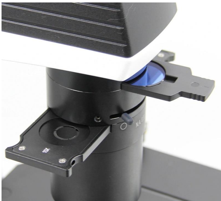
Filters: Blue, Dia.34mm; Green, Dia.34mm
